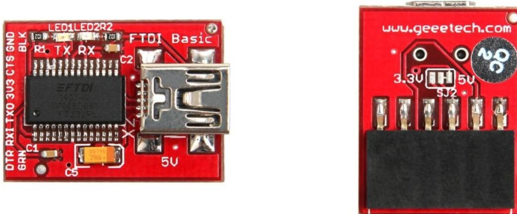
Photos 2A and 2B. Example 6-pin USB adapter.
