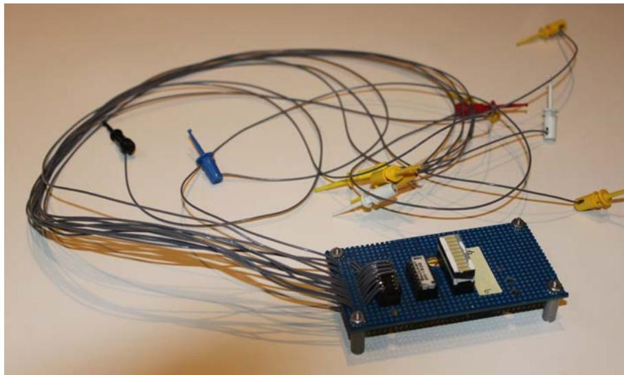
Indicator LEDs with detachable clip leads to circuit
