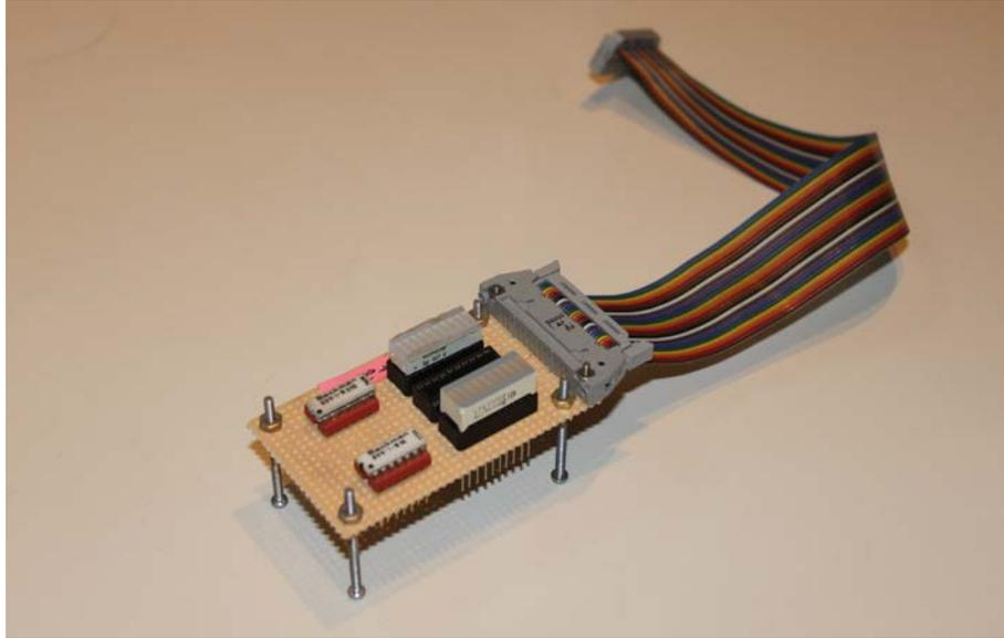
Indicator LEDs with cable headers to circuit IO
